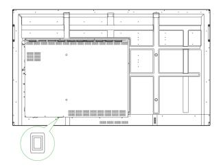
3. Press the power button on the display or the remote control to power on the display.
