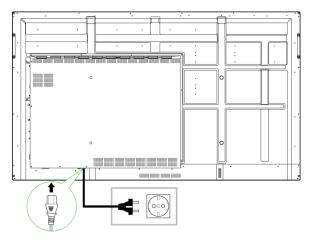
2. Turn the power switch located at the bottom of the display on.
