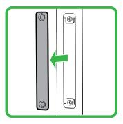
3. Insert the OPS module into the slot.
