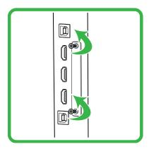
2. Remove the Wi-Fi module slot cover.
