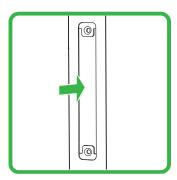
4. Install the two screws to secure the OPS module to the display.
