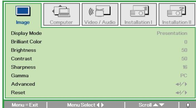
2. Press the cursor ←→ button to move to the **Installation I** menu, press the cursor ↑↓ button to select **Advanced**.
