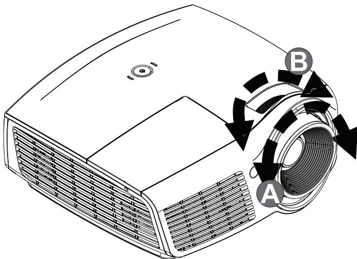
2. Use the **Image-focus** control (on the projector only) to sharpen the projected image **A**.
