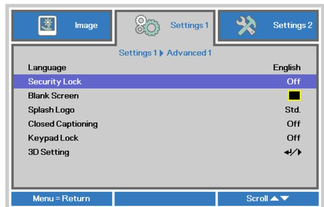
5. You can use the cursor buttons ▲▼◀▶ either on keypad or IR remote control for password entry. You can use any combination including the same arrow five times, but not less than five.
